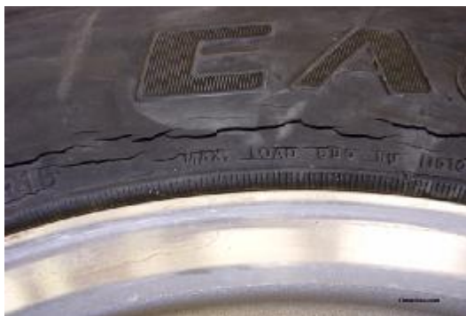
Figure 2.2 Sidewall with ozone cracks.
